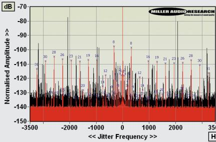
**ABOVE:** High resolution 48kHz/24-bit jitter spectrum (S/PDIF, black and via USB, red with markers)
