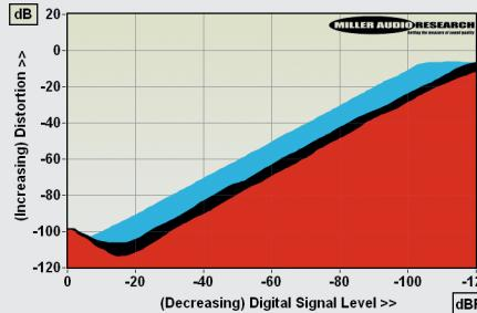
**ABOVE:** Distortion versus 48kHz/24-bit digital signal level over a 120dB dynamic range (via USB, 1kHz, red infill; via S/PDIF, 1kHz, black; 20kHz, blue)
